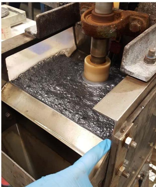
Figure 1: Lead (Pb) rougher-cleaner flotation testwork – up to 79% Pb
