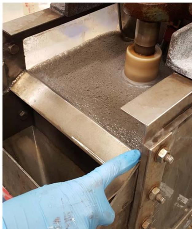
Figure 2: Zinc (Zn) rougher-cleaner flotation testwork – up to 58% Zn
