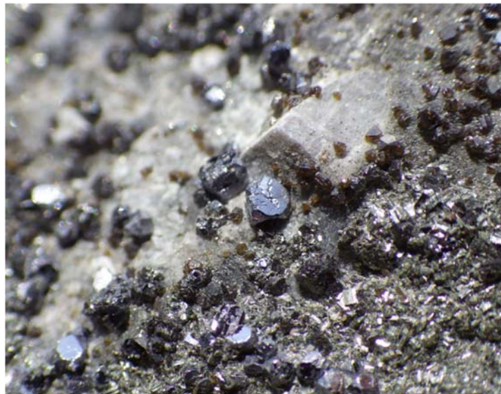
Figure 1: Very coarse, crystalline galena and sphalerite in a section of core from hole DKDD001
